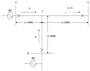
The Zone 2 reach is obtained by adjusting the impedance setting.
