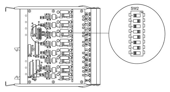
Note: Switch SW2 controls 8 status inputs. As supplied, all switches are in the left hand position and all status inputs are high speed devices
